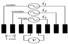
Fig: 6. Electrode Array with Three Alternative Current Injecting Electrode Sets and one Set of Voltage Pickup Electrodes
