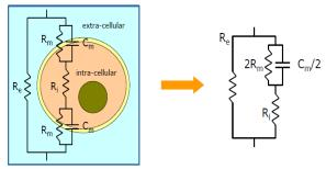
Fig: 1. Equivalent Circuit of a Cell
