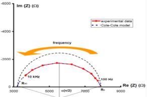
Fig: 3. Wessel diagram of an actual bioimpedance measurement and the superimposed Cole model results.
